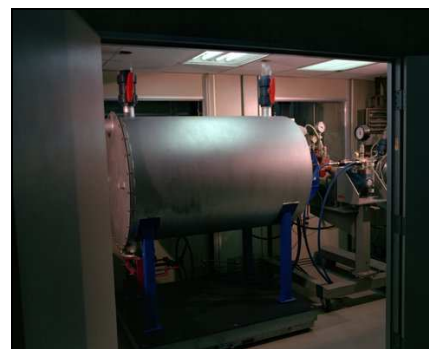
Fig 40. Right: community support for anaerobic digestion. Left: an anaerobic processing unit. Anaerobic digestion can reduce green greenhouse gas emissions by capturing methane from the decomposition of organic materials, such as livestock manures and slurries, sewage sludge and food wastes
